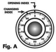
TO LOCK: Close the door and turn the handle. Turn the dial to the LEFT (counter clockwise) at least 4 full revolutions.
